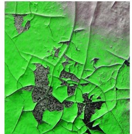
Underlying paint shows severe cracking due to solvent attack from the graffiti
