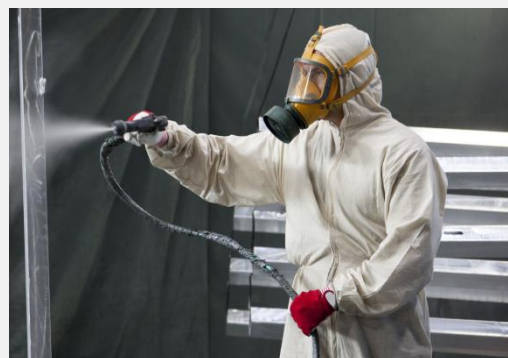
In spray shops, correct personal protection equipment keeps the applicator safe from inhalation of spray mist and solvent vapour
